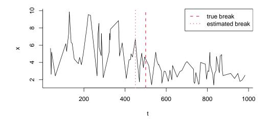
The likelihood is used to obtain a BIC value for all of the possible models. The possible models are numbered M0 to M7, corresponding to no significant changes (M0), only  $\mu$ ,  $\sigma$  or  $\rho$  changing (M1, M2, M3, respectively), both of  $\mu$  and  $\sigma$ ,  $\mu$  and  $\rho$  and  $\sigma$  and  $\rho$  changing (M4, M5, M6), and all three parameters changing (M7). The model are compared with the GetModels function:
