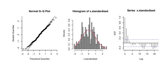
This plot illustrates the qq-norm plot, the histogram and the auto-correlation function of the standardized data  $(Z_i = X_i - \hat{\mu}(T_i)/\hat{\sigma}(T_i))$ . Overall the results seem to satisfy the assumptions of normality.
