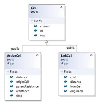
Figure 2: Schematic representation of Cell type data structures.
