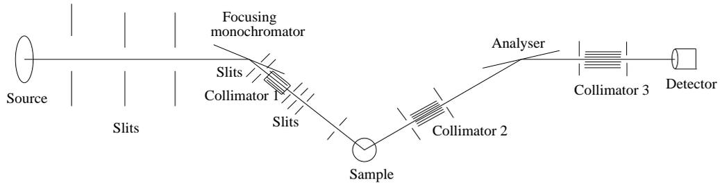
Figure 8.3: A sketch of the TAS1 instrument.
