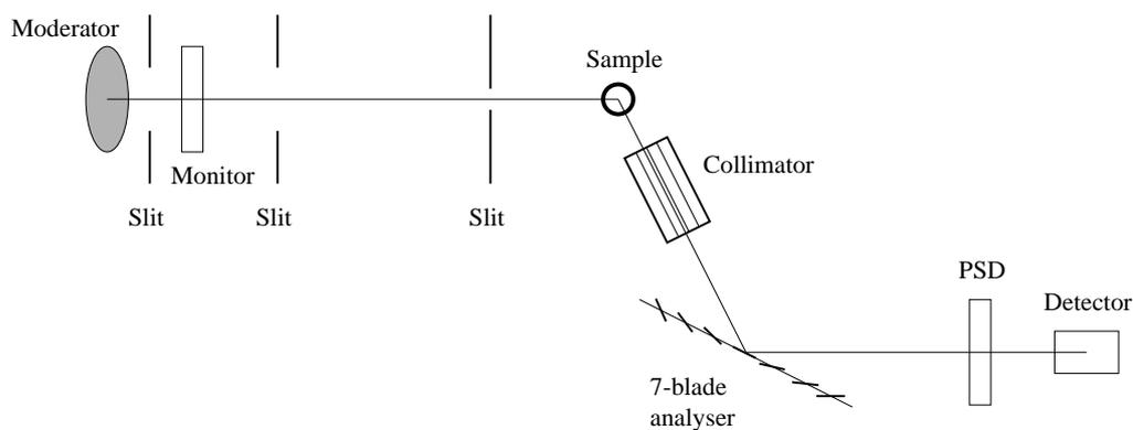
Figure 8.8: A sketch of the PRISMA instrument.
