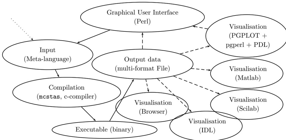
Figure 5.1: An illustration of the structure of McStas .
