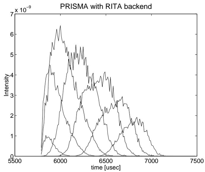
Figure 8.9: Test result from PRISMA instrument using “colored neutrons”. Each graph shows the neutrons scattered from one analyser blade.
