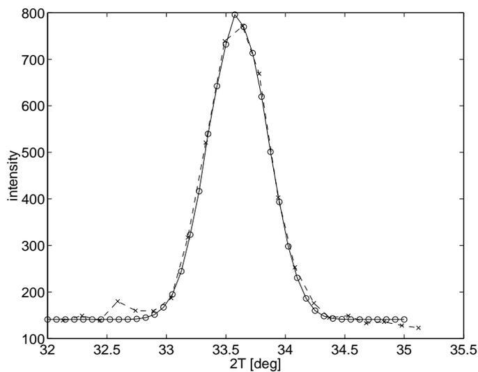
Figure 8.6: TAS1:  $2\theta_s$  scans on  $\text{Al}_2\text{O}_3$  in two-axis, focusing mode. Collimations: open- $30^\circ$ - $28^\circ$ - $67^\circ$ . "x": measurements, "o": simulations. A constant background is added to the simulated data.
