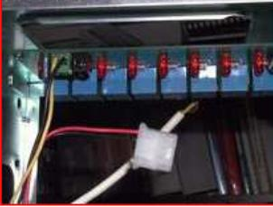
This shows the 12V connection to the relay board. I mounted it from the top of the cabinet, and the 12V input is from the computer power supply.
