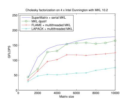
Figure 1.3: Performance of Cholesky factorization implementations measured on a 24 core Intel "Dunnington" system. Theoretical peak system performance is 255 GFLOPS. libflame uses variant 3 while LAPACK uses variant 2. For non-SuperMatrix experiments, MKL was invoked in multithreaded mode. For SuperMatrix experiments, MKL parallelism was disabled. Blocksizes were tuned individually for each problem size tested.
